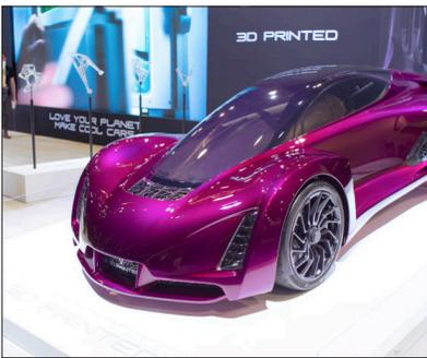
**Divergent 3D's Blade** is a proof of concept vehicle, showing it is possible to build whole cars (except the carbon fiber reinforcements, wheels, and tires) out of 3D printed metal.
