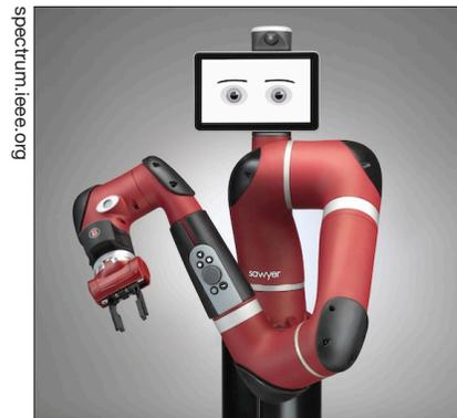
The user-friendly robot **Sawyer** learns by a human grabbing hold of its wrist and leading it through an activity once. Its series elastic actuators give it a high level of accuracy in sensing forces, enabling it to take on more delicate tasks.
